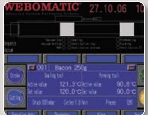
12" colour touch screen for visual process monitoring and direct setting of parameters of the PLC.
