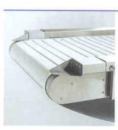
It is possible to reduce the tension of the belt for the cleaning process. The belt's tension is regulated pneumatically. The picture shows the optional special belt for round products.
